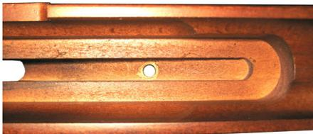
Countersink hole to allow screw to sit flush.
